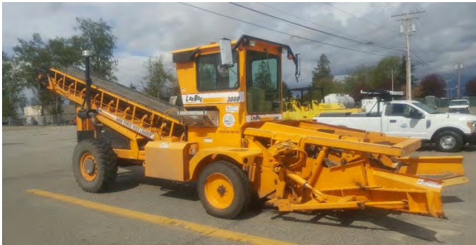
Sod Picker used to transfer windrows of sod and gravel into dump trucks
